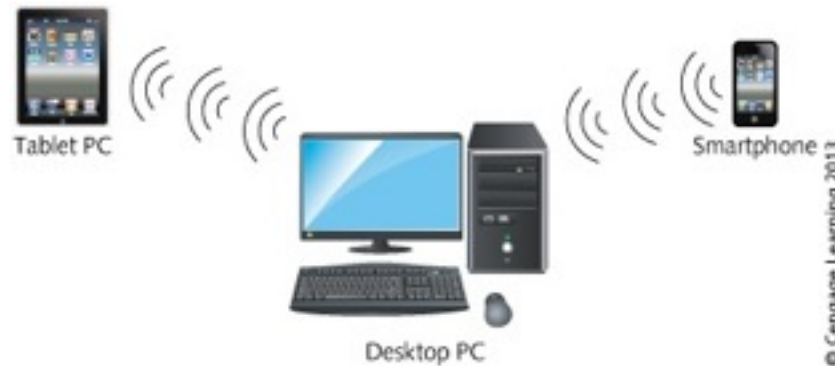
Figure 1-3 A desktop PC, a smartphone, and a tablet PC forming a PAN
